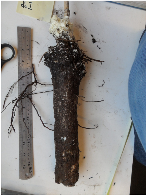
Figure 11: Extracted foam core with trapped root ends from Hallyburton Hill
