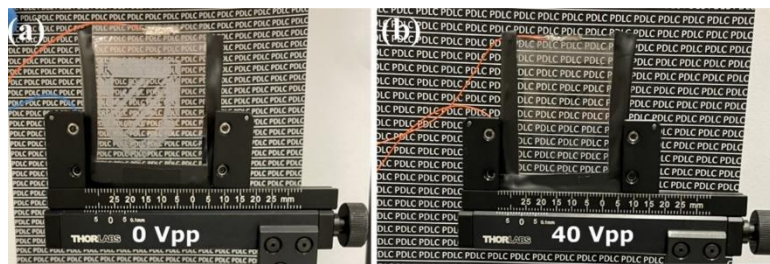
Figure 5.4 Patterned PDLC logo with (a) 0 Vpp applied and (b) 40 Vpp applied.
