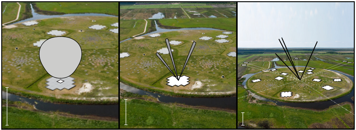
Figure 3.1: Image and caption taken from Stappers et al. (2011). Three successive zoom-outs showing the stations in the LOFAR core. The different scales of the hierarchically organised HBA elements are highlighted and their respective beam sizes are shown. The large circular area marks the edge of the Superterp, which contains the inner-most 6 stations (i.e. 12 HBA sub-stations: where there are 2 sub-stations, each of 24 tiles, in each HBA core station); other core stations can be seen highlighted beyond the Superterp in the third panel. Left: a single HBA tile and associated beam. Middle: A single HBA sub-station with three simultaneous station beams. Right: The 6 stations of the Superterp plus 3 core stations in the background are highlighted. Four independent beams formed from the coherent combination of all 24 core HBA stations, most of which are outside this photo, are shown.
