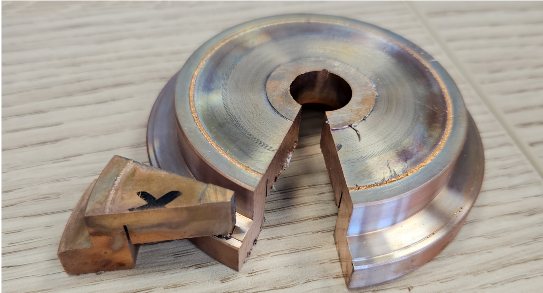
Figure 2.21: Initial test of EBW on a similar geometry to the cavity body and endcap. The cut-out cross-section shows excellent weld penetration.
