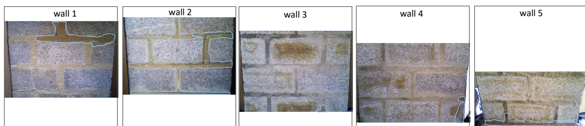
Figure 6.12. Visual comparison of the back of the test walls after spraying and after 6 hours of evaporation ( t=6 h). The blue boundaries highlight the egress of moisture. Missing parts of the walls are due to the location of the camera, but most of the moisture pattern are shown here.
