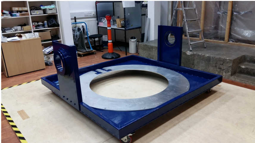
Figure 12 WEAVE Handling and assembly trolley with positioner baseplate.
