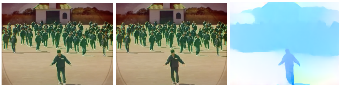
Figure 1.1: Object emerges from motion. In the first two images, we show two neighbouring frames from the series Squid Game . The players (in green) were playing a children’s game where they get eliminated if they move. The character in front moves only slightly, but the optical flow (right image) clearly highlights the motion. From Squid Game , Season 1, Episode 1: Red Light, Green Light .
