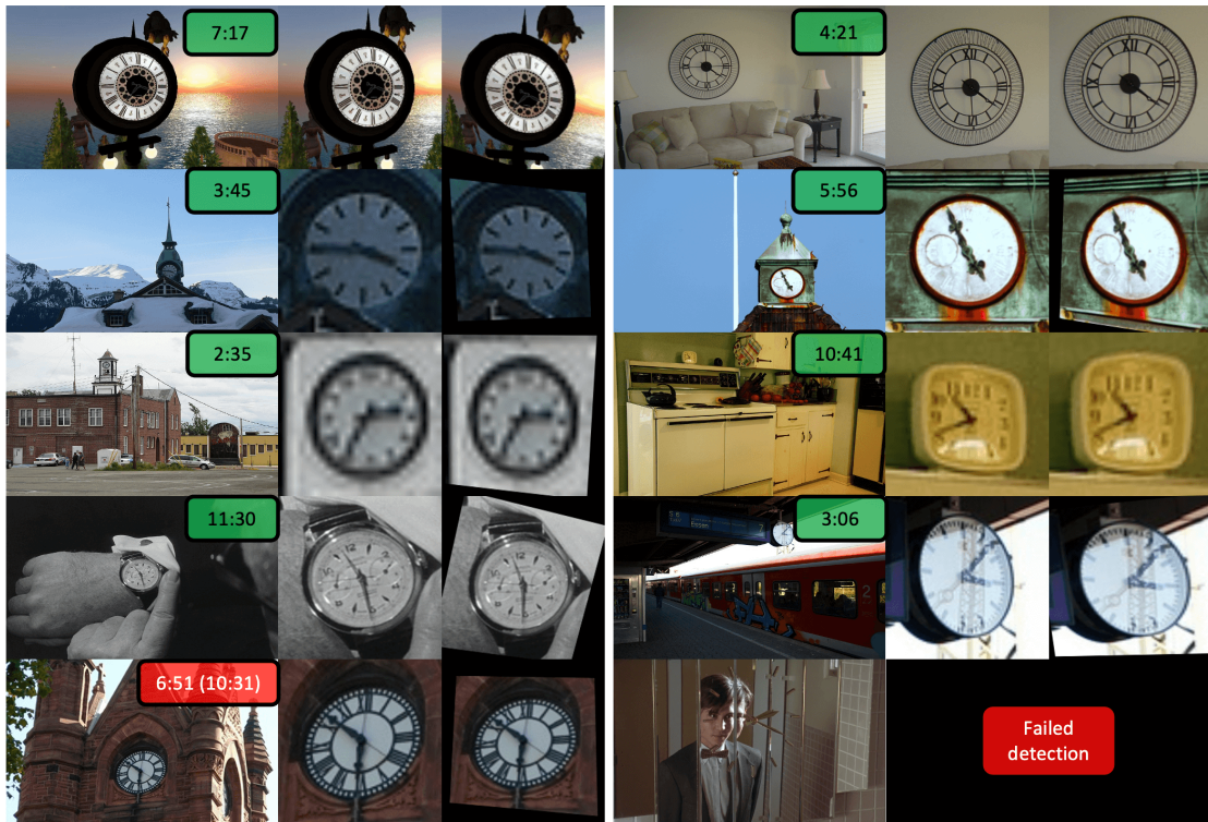
Figure 5.6: Qualitative results. The columns show the original, cropped, and canonical images, with predicted time overlaid on the original image. The model is able to read clocks in varying and challenging scenes, including those with different styles (rows 1-2), low resolution (row 3), and non-frontal viewing angles (row 4). The bottom row shows two failure cases: reading swapped hands and failed detection.
