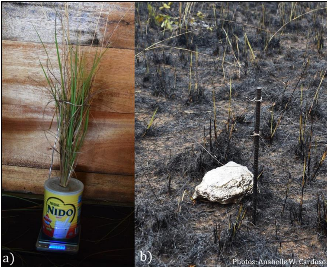
Figure 4.3: a) An example of the simple apparatus used to measure flammability traits of the grass species, this image shows the set up to measure maximum combustion rate, whereby a piece of grass is burnt and the speed at which it loses weight is recorded. b) One of the thermocouples used to measure fire intensity and temperature, the data logger was wrapped in a fire blanket and aluminium foil, leaving only the thermocouple wire outside, which was attached to a metal rod at 30 cm above the ground.
