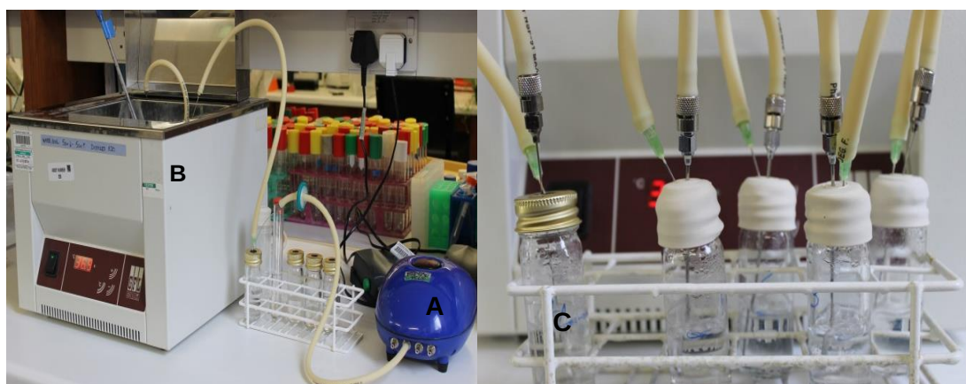
Figure 2.2: Mini-reactor set up for aerobic growth condition. Fish pump (A) was used to sparge air into the cultures and the water bath (B) maintained a growth temperature of 37°C. The cultures were connected to humidifiers (C).
