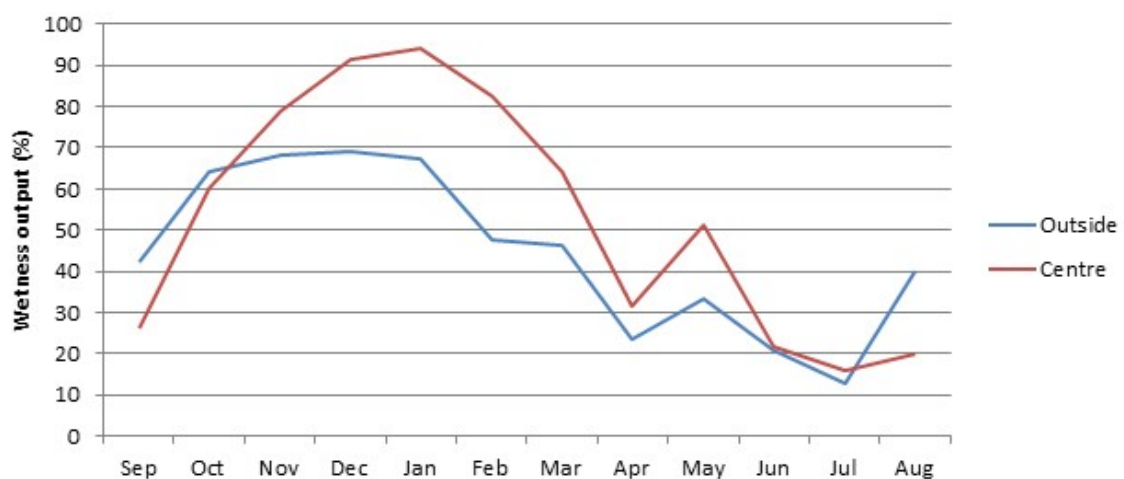
Figure 5.16: Monthly means of daily mean wetness occurrence (%) outside and in the centre of the shelter
