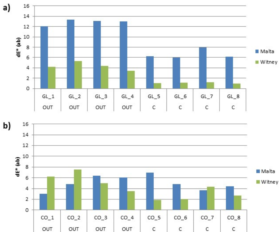
Figure 9.8: Overall colour difference (dE*ab) in a) Globigerina and b) Coralline samples located outside (OUT) and in the centre of the shelter (C) in Malta and at Witney after a year of exposure
