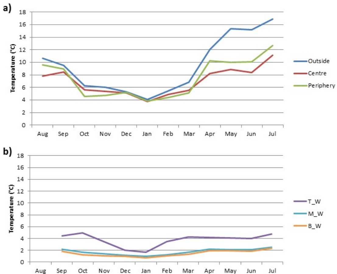
Figure 5.8: Mean of diurnal temperature difference per month (a) outside, centre and periphery of the shelter and (b) at the different parts of the wall (T_W= top part of the wall; M_W=middle part of the wall; B_W= bottom part of the wall)
