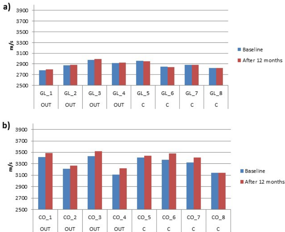
Figure 9.6: Median of the UPV values in a) Globigerina and b) Coralline samples located outside (OUT) and in the centre of the shelter (C) in Malta before and after a year of exposure
