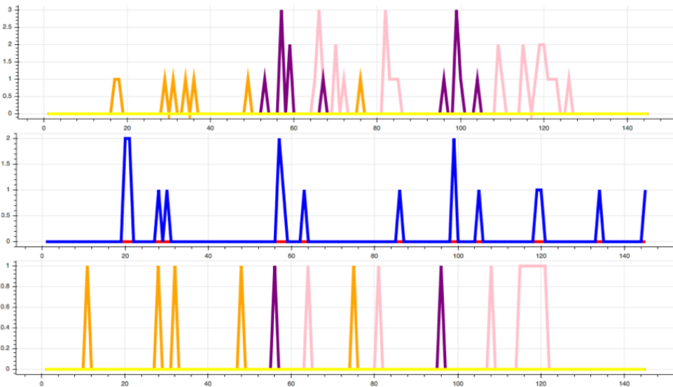
Figure 9.2: Dataset 2 network-traffic awareness: true-positive detections (top); false-positive and unidentified detections (middle); ground truth (bottom)
