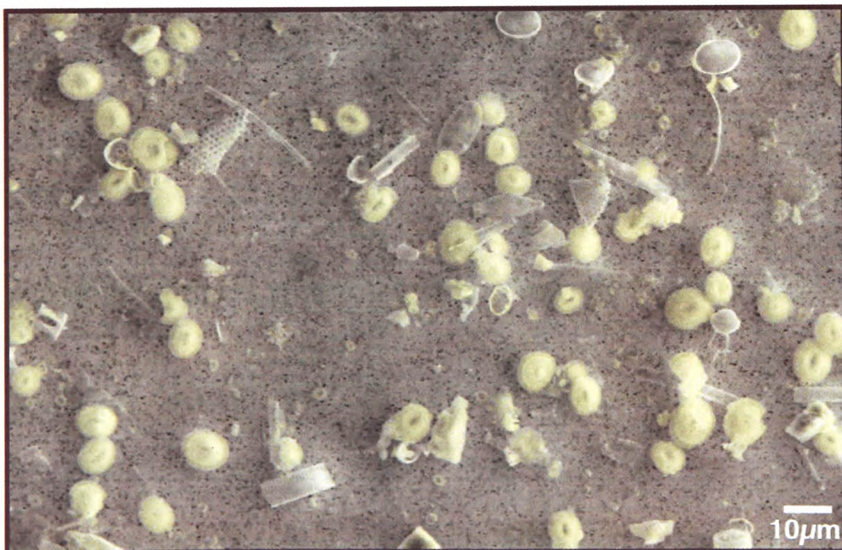
Figure 7. Scanning Electron Micrograph (SEM) image of < 10 \mu\text{m}</math> filtered sediment of RAPID 21-12-B core-top. The image has been overlaid with a Ca map to highlight \text{CaCO}_3 material. It is evident that coccoliths dominate the \text{CaCO}_3 material. Note; SEM image taken at filter edge skewing population.
