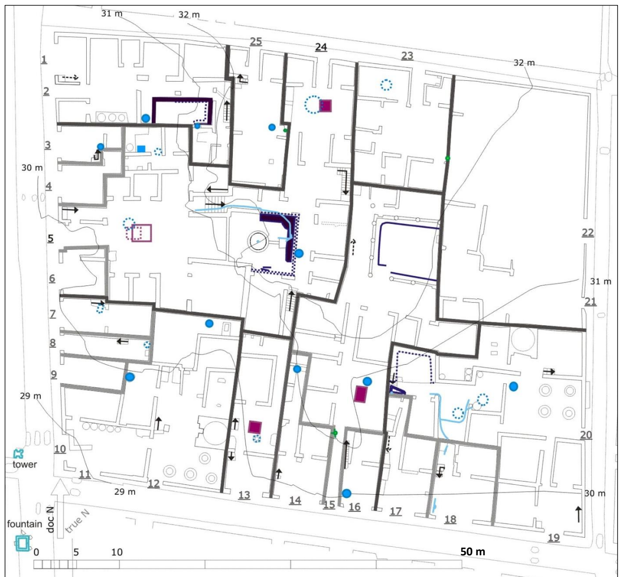
Figure 39. Water supply structures in insula IX.3. The close-by water tower and public fountain are also marked, as are contour lines (m ASL). A probable impluvium under repair in Room 2 is outlined, structures out of use in AD 79 are marked with a broken line and those most probably in use are coloured in full. Unit borders are shown in mid-grey, hypothetical property borders are highlighted in black.
