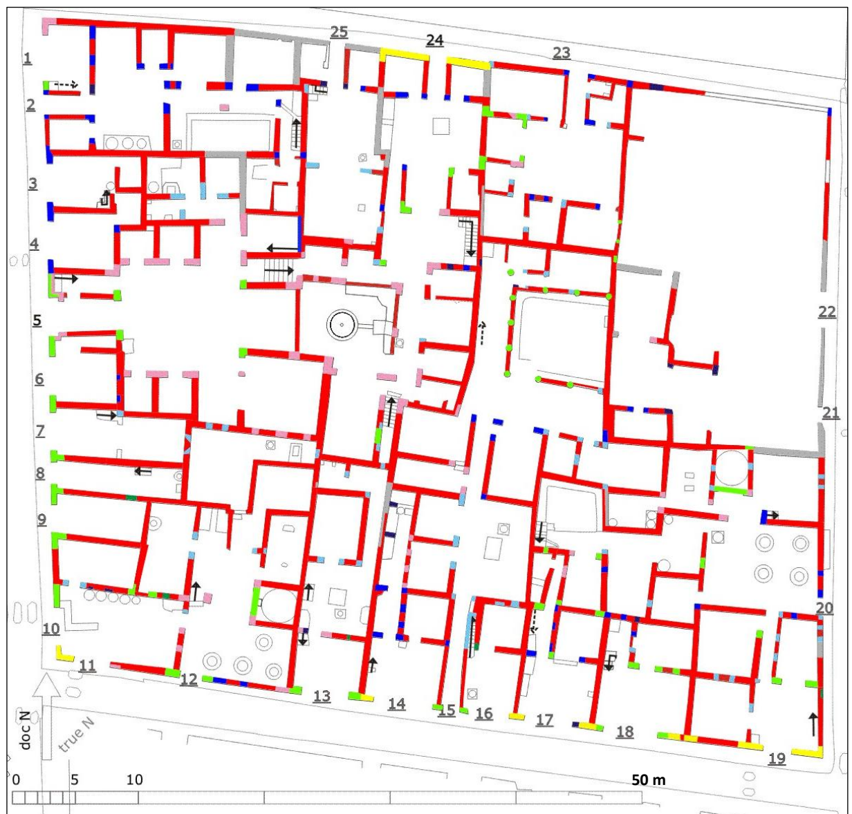
Figure 59. The approximate distribution of different wall construction types in insula IX.3 .
