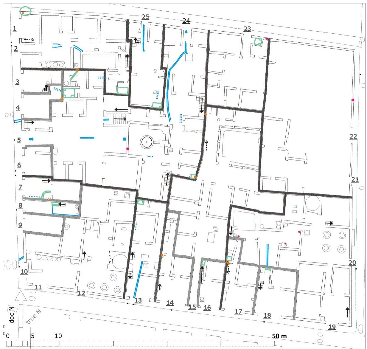
Figure 52. Drains and toilets in insula IX.3. Structures out of use in AD 79 are marked in broken lines. Unit borders are shown in mid-grey, hypothetical property borders are highlighted in black.
