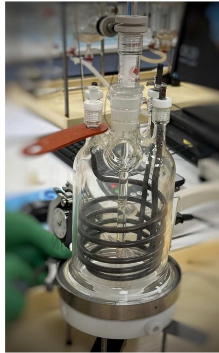
FIGURE 3 | Left: sketch of the CPT test cell adapted from the ASTM G150 standard [34], and right: the actual used AVESTA cell. [Color figure can be viewed at wileyonlinelibrary.com ]
