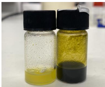
Figure 4-13 DMA (75 mM), LiTFSI (0.1 M) in tetraglyme with excess KO 2 after 1 hr mixing (yellow) and 8 hr mixing (brown) suggesting that superoxide reacts with DMA.
