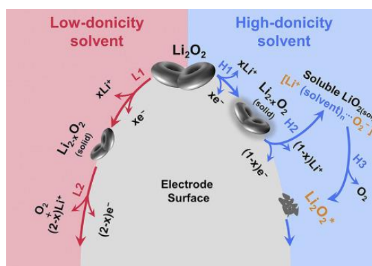
Figure 1-8 Schematic representation of the effect of the donor number of the solvent on the charge process. Reprinted with permission from ref 68. Copyright 2018, Elsevier.
