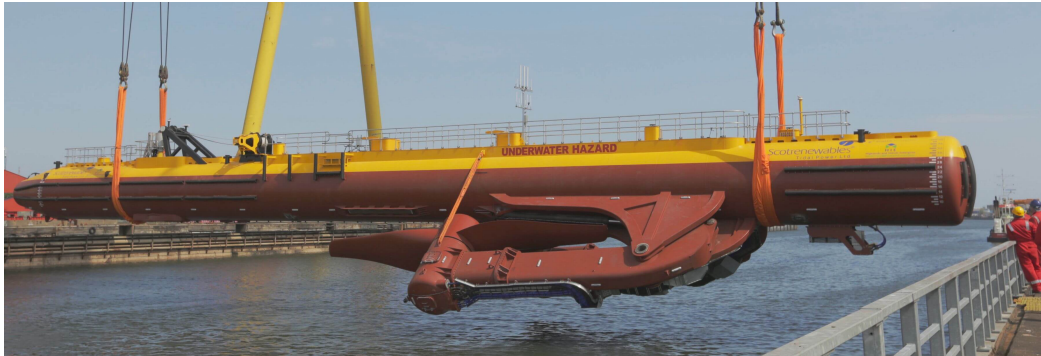
Figure 1.4: Deployment of ScotRenewables’ SR2000 dual-turbine floating generator (Image reproduced with permission of Scotrenewables Tidal Power Ltd.)
