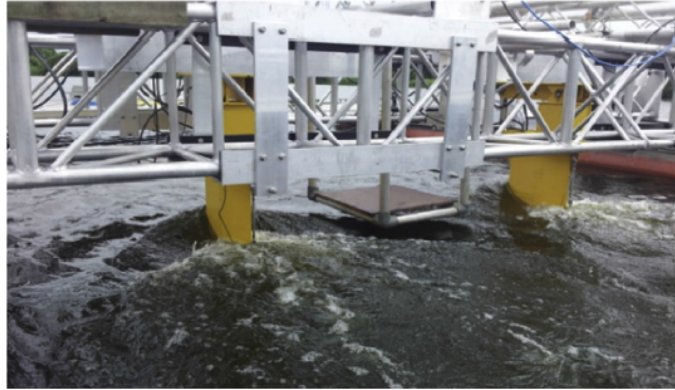
Figure 2.8: Support structure for two scale rotors being tested side-by-side in open water. (Image reproduced from Jeffcoate et al. 2016 [61] with permission of Elsevier.)
