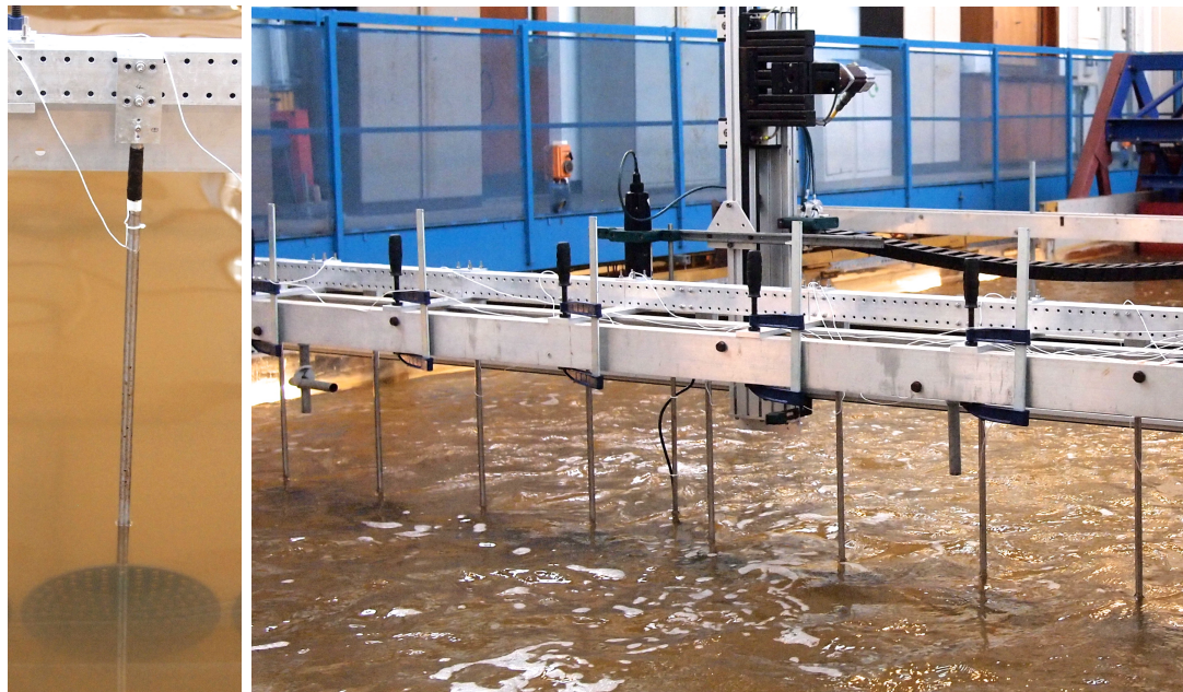
Figure 5.3: Photographs of: a) a single disc and its support tower, seen from downstream of the array. Strain gauges are mounted under the black protective coating at the top of the tower; b) disc array seen from upstream of the array. ADV traverser equipment and probe support can be seen behind the array.
