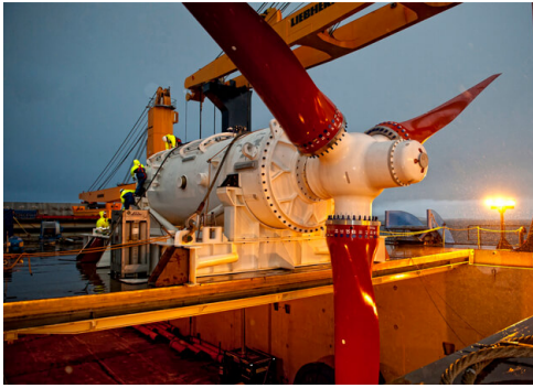
Figure 1.6: HS1000 prototype turbine (Image reproduced with permission of Andritz Hydro Hammerfest.)
