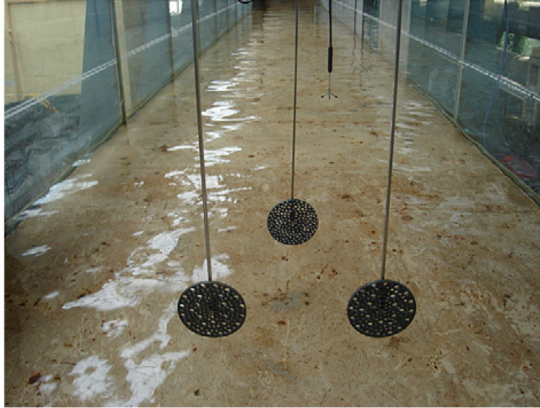
Figure 2.7: Experimental set-up of three porous discs in a staggered, two-row configuration. (Image reproduced from Myers et al. , 2011 [86] with permission of Elsevier.)
