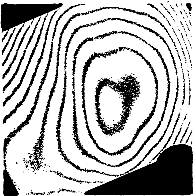
Figure 2.9 Interferogram of float glass substrate (633 nm)
