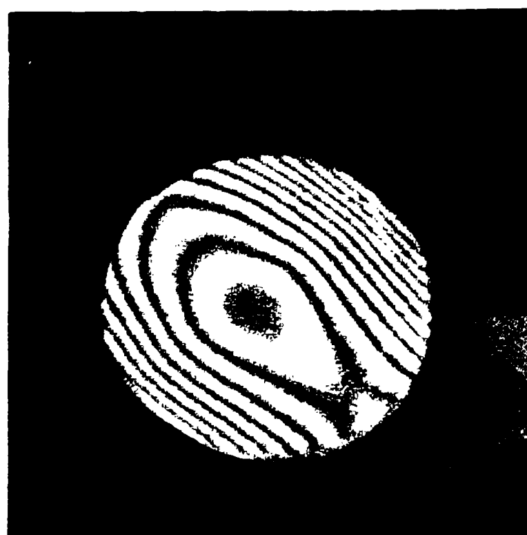
Figure 2.16 Diffraction using float glass substrate - with coverplate (514.5 nm)
