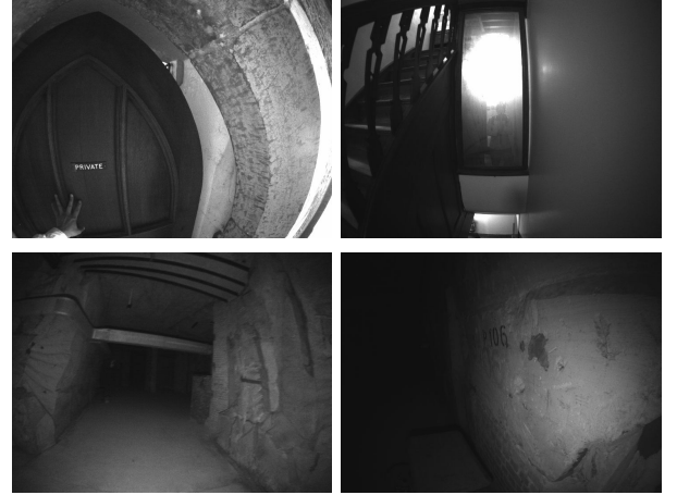
Fig. 7. Visual challenges in the NCD-Multi Dataset. Top Row : Images from NCD-Multi Stairs sequence with door opening (obscuring the cameras) shown on the left. On the right is a tight space about 1.5 m wide and a mirror. Bottom Row : Images from NCD-Multi Mine sequence with darkness and the challenge of camera being held up close to a wall.
