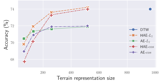
Fig. 6: The terrain recognition accuracy for the unsupervised, compressed tactile signals depends on the latent vector's length (representation) used to capture the original properties of the F/T signals
