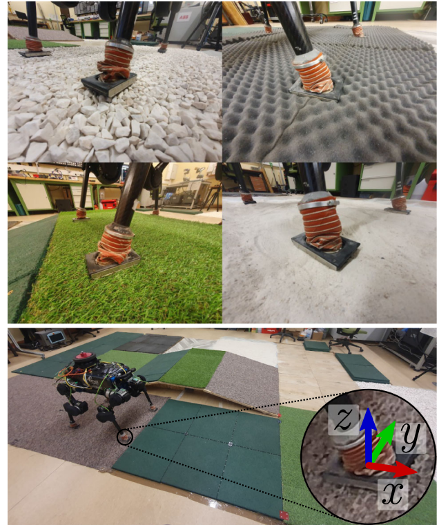
Fig. 10 Top: Examples of foot positioning when collecting data on different terrains under controlled laboratory conditions. Bottom: Experiment 3: ANYmal with sensorized flat feet standing on the multiple terrain type course. Close up of the foot is provided. An IMU and fore/torque sensor is located in the sole with coordinate frame shown
