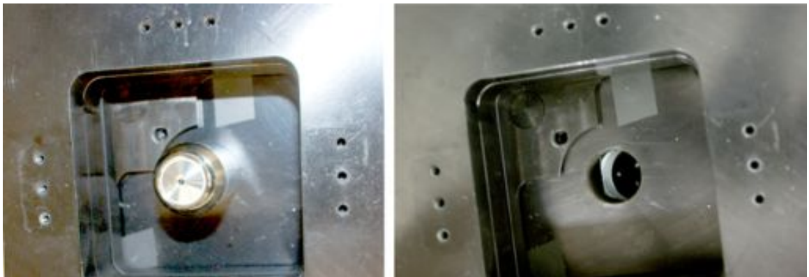
Figure 2.8: Two photographs looking down onto the stage. The image on the left shows the objective in place, and the image on the right shows the objective removed, with the 45° mirror visible. Illumination light passes through the 1mm hole in the mirror, which is visible. A second hole is also visible; the hole lies outside the area illuminated by backscattered light, and thus does not affect the mirror's performance.
