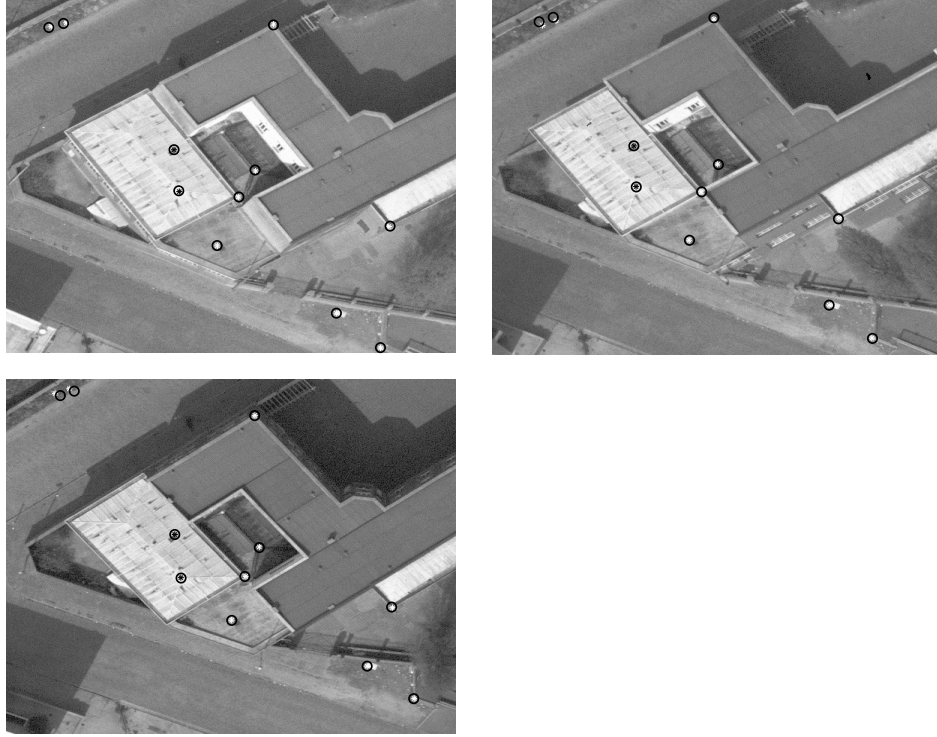
Figure 2: Reprojection errors of the eleven points. The data points are marked with "*" and the reprojection points with "o".
