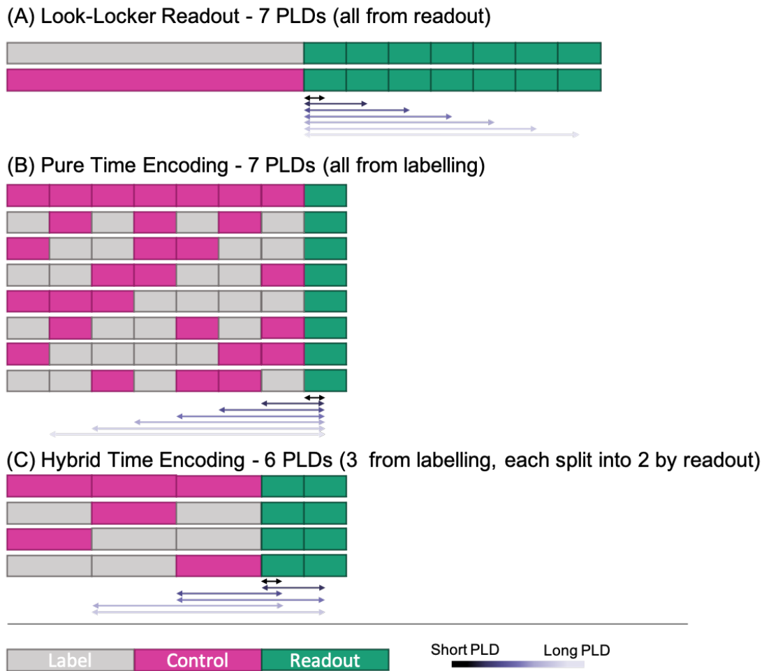
Figure 5.1: Three different approaches to achieving dynamic ASL imaging. The purple arrows between the ends of the labelling blocks to the centre of the readout blocks depict the PLDs.
