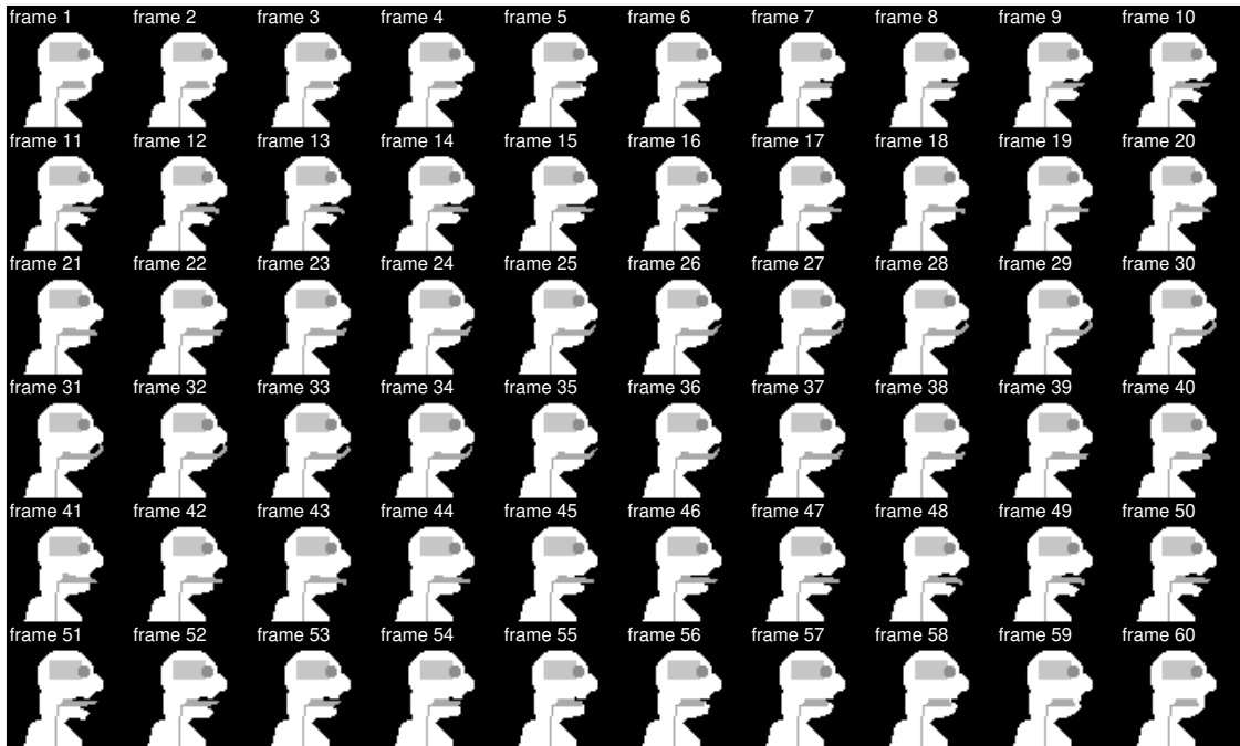
Figure 6.3: Dynamic phantom used for SILVER experiments. It is temporally symmetric with the first 30 frames being reversed in the last 30 frames. The "tongue-like" and "jaw-like" structures move between frames, everything else is stationary.
