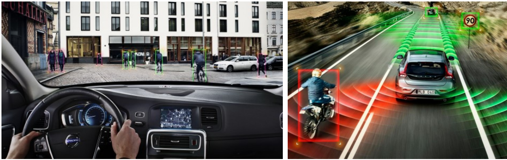
Figure 1.3: The Volvo S60 uses pedestrian and car detection systems for warning the driver and even makes full power auto break decision in order to avoid an accident. Photo courtesy Volvo, Sweden.
