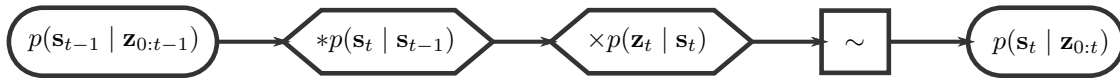
Figure 6.1: Filtering diagram for the basic particle filter following the convention of MacCormick et al. [175, 176]. The round edged boxes represent distributions in the form of particle sets. The hexagonal boxes represent operations on each particle in the particle set: the ‘*’ represents convolving the particle set with the state evolution distribution and the ‘x’ represents multiplying the particle weights by the measurement distribution. The square box containing the ‘~’ represents the resampling operation across the entire particle set.
