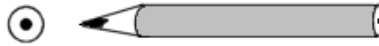
Figure 1.1 – Example of 'hidden' information. A pencil viewed from head-on contains no information about the pencil's length, when viewed at a 90-degree angle the length is now measurable.
