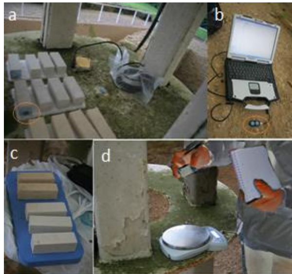
Figure 7: Small blocks are used for experimental investigation of rock weathering in a heritage conservation project. The data loggers (recording humidity and temperature) are circled (a and b). Once the data is downloaded the samples are weighed (c and d) (Images digitally altered to protect anonymity of participants using Zoner Photostudio 15)
