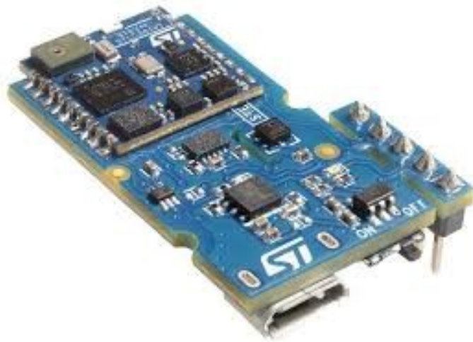
Figure 3.1: A STEVAL-STLKT01V1 development board
