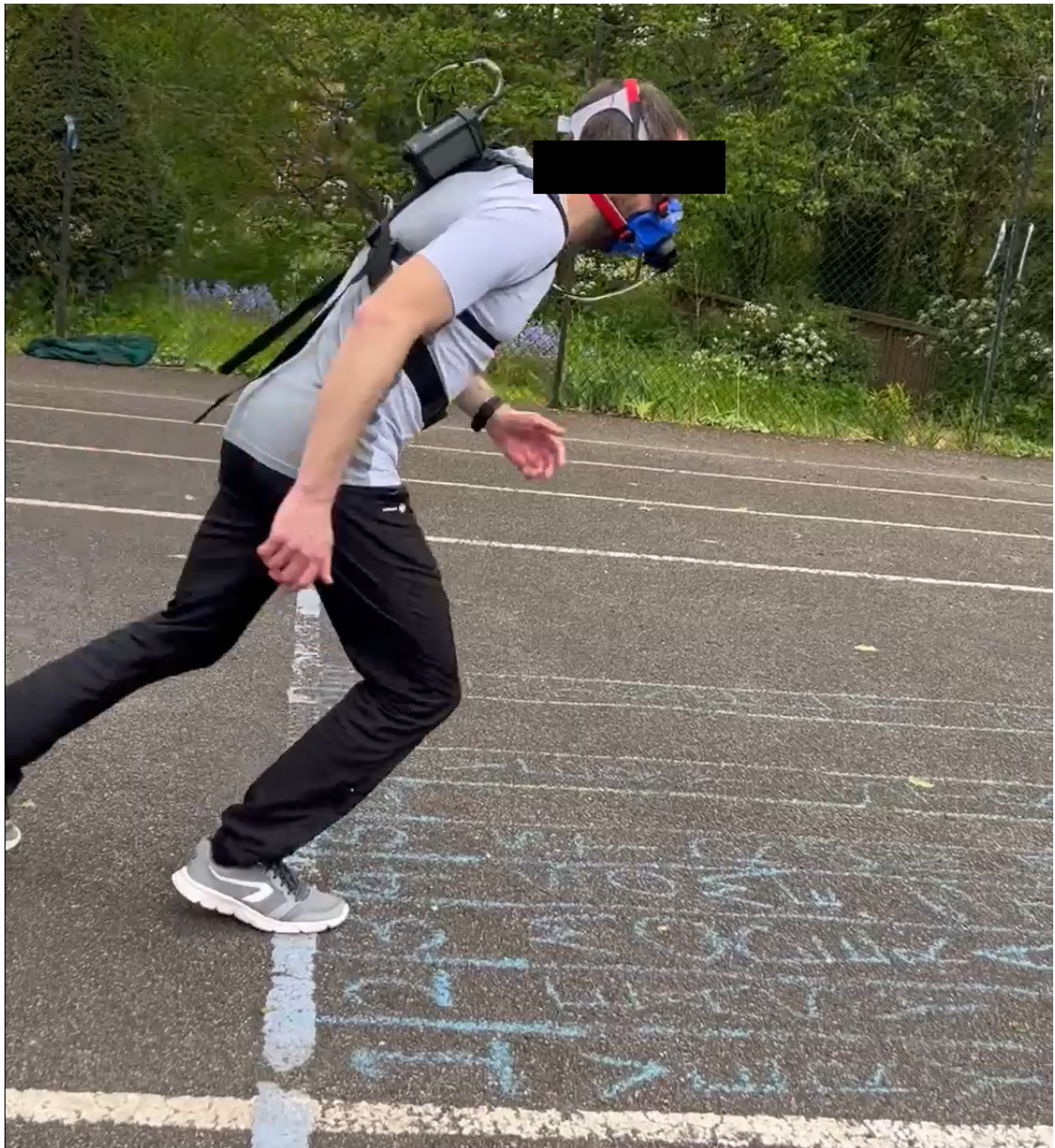
Figure 4.3: This figure shows a participant, wearing the COSMED K5, a Polar H10 heart rate strap, and a microphone-instrumented mouthguard, at the starting (0m) line at the beginning of a Yo-Yo test level. The Borg CR10 RPE scale, written in chalk, was marked in front of the start (0m) line. The participant can be seen stepping on the number 3, indicating their RPE level was 3 at that instant.
