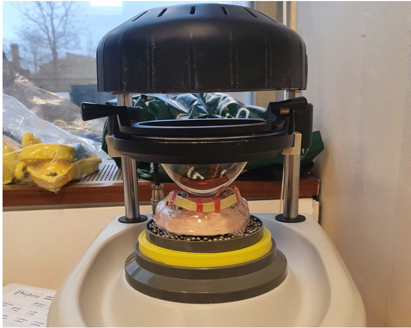
Figure 3.14: This is an example of the thermoforming process. In this image, the electronics have already been assembled onto the mouthguard's base-layer, and the outer-layer is about to be vacuum-formed over the assembly.
