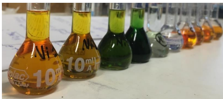
Figure 38 The samples used for the Stern-Volmer studies displayed a range of colors from orange ( [\text{Ru}(\text{bpy})_3]\text{Cl}_2 \cdot 6\text{H}_2\text{O} 200 \mu\text{M} only) to dark green ( [\text{Ru}(\text{bpy})_3]\text{Cl}_2 \cdot 6\text{H}_2\text{O} 200 \mu\text{M} + [\text{NiCl}_2(\text{PPh}_3)_2] 125 \mu\text{M} ).
