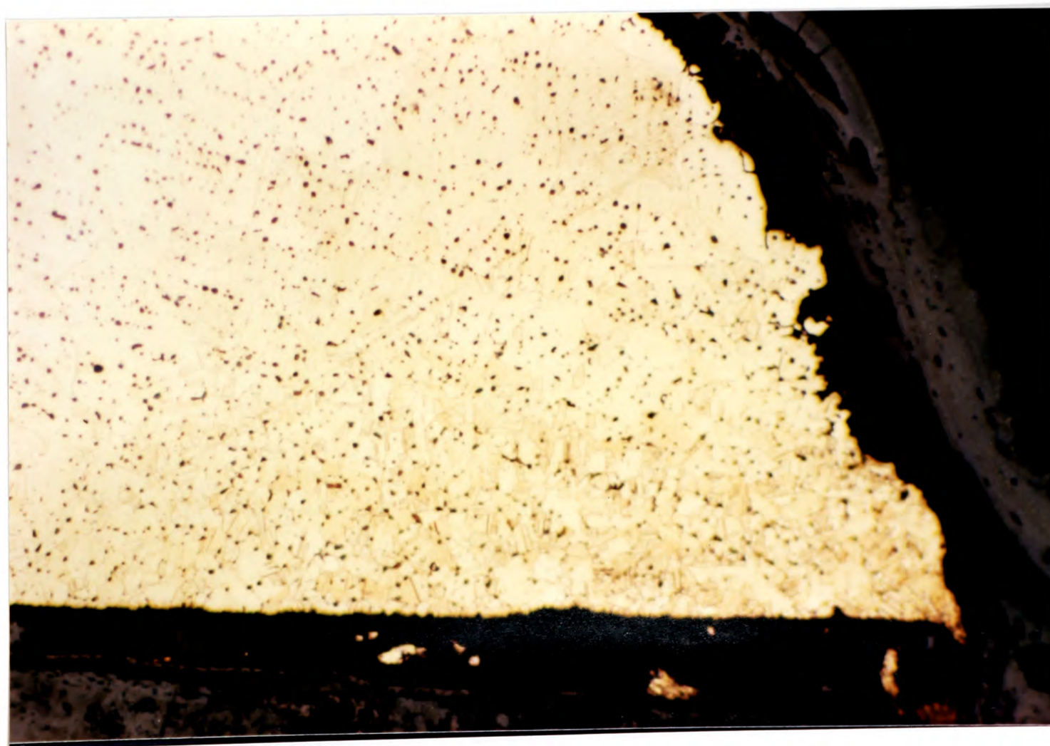
Plate 9 Ditto, showing crystal structure (recrystallisation) x100
