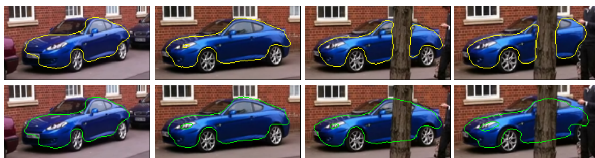
Figure 6.6: Example frames from a video tracking a car, comparing our method to the PWP tracker of [13]. When the car is not occluded both methods produce similar results. When the tree is in front of the car the segmentation produced by the PWP tracker is corrupted, while the one produced by our tracker is not.
