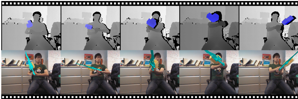
Figure 3.7: Film strips from a whole tracking sequence. The top row shows the observed depth with object overlay, while we show the tracking result with graphical visualization with a virtual sword on the lower row. Whole sequence see Video B.1 in Appendix B .
