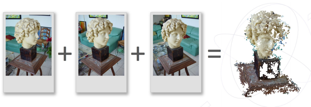
Figure 2.11: Example result of SfM-based reconstruction. Image from Xiao [146]
