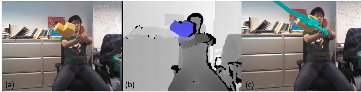
Figure 3.1: Illustration of the concept of control object tracking. Image (a) shows the original colour image, (b) shows the depth image with tracking result overlaid, (c) visualizes a sword on the colour image with the recovered pose of the control object.
