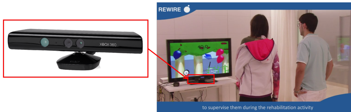
Figure 1.2: The Kinect sensor (left) and the setup of patient station of home rehabilitation platform (right).
