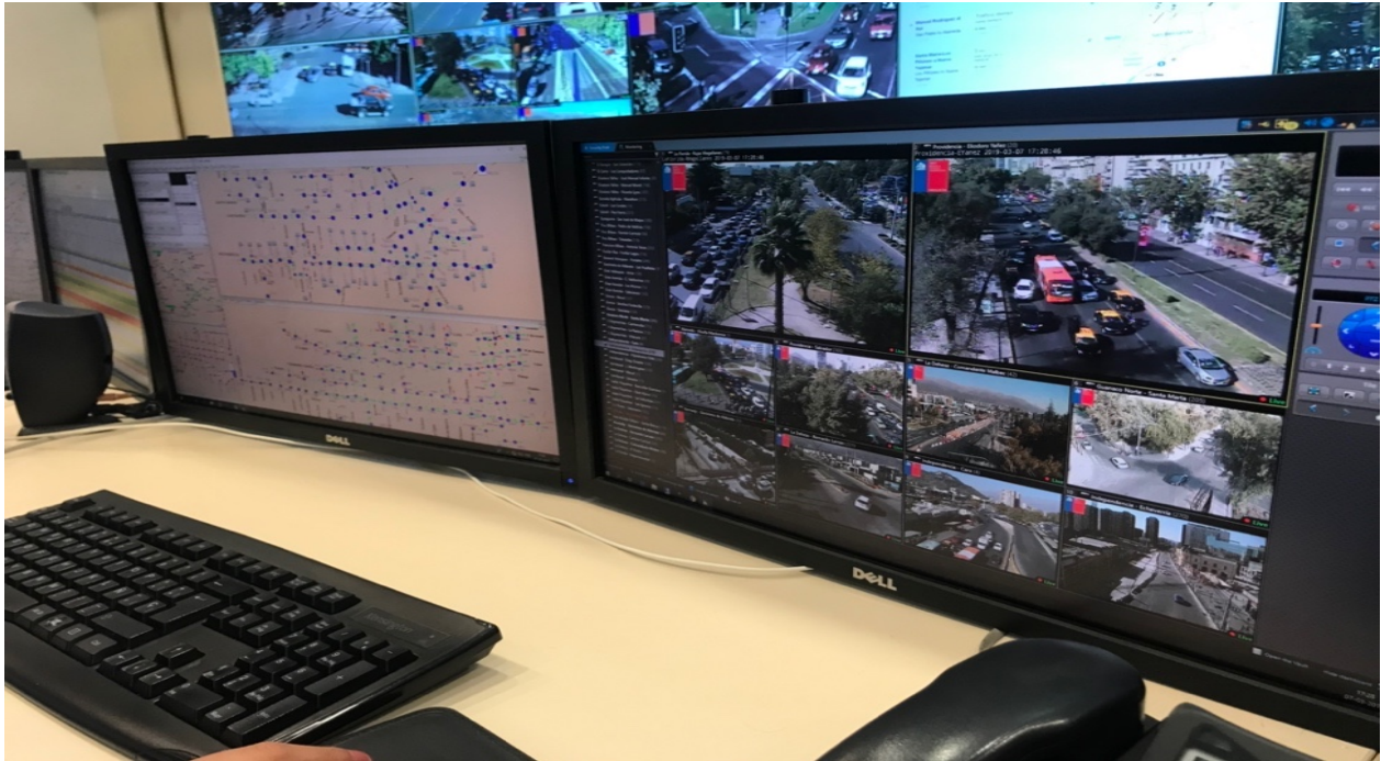
Figure 12. UOCT Analyst desk setup. Left screen shows the SCOOT software layout of dynamic control traffic management. Right screen shows specific CCTV images selected by the analyst. (Ignacio Pérez, participant observation, 2019).
