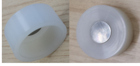
Figure 7.16: Anvils: tungsten cores inserted into nylon cups
