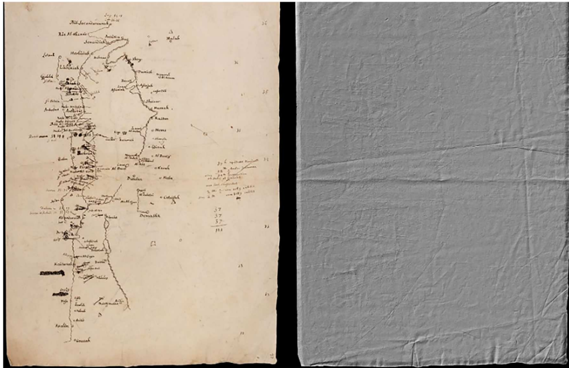
Fig. 2. A 3D recording of an eighteenth-century manuscript map of the Middle East by John Gagnier in true colour (left) and a shaded surface render (right). The image reveals scoring on the map's surface which is not otherwise visible, providing insights into the map's creation (Map Res. 73; © Bodleian Libraries, courtesy of ARCHiOx/John Barrett).
