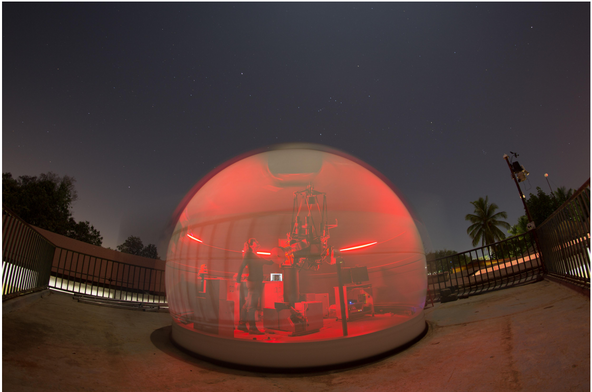
Figure 3.4: View of the inside of the GJW-IN dome. The red light (switched off during observations!) helps to maintain dark adaption in the operator's eyes. This photo was taken by Steve Lee.
