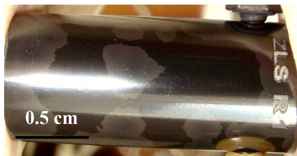
Figure 4.3 A patchy oxide formed on ZIRLO SR material after 140 days.
