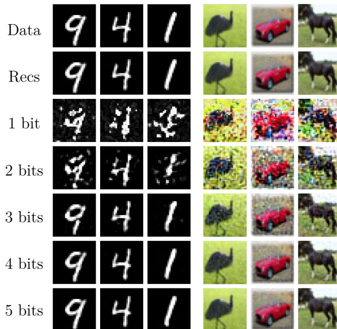
Figure 4.15: Qualitative effects of quantization. The top row shows ground truth data from MNIST and CIFAR10, the second row shows the reconstructions from full precision (32 bit) modulations. The subsequent rows show reconstructions when quantizing to various bitwidths. As can be seen, with only 5 bits, reconstructions are nearly perfect. Using as few as 1 or 2 bits, the class of the object is generally recognizable.
