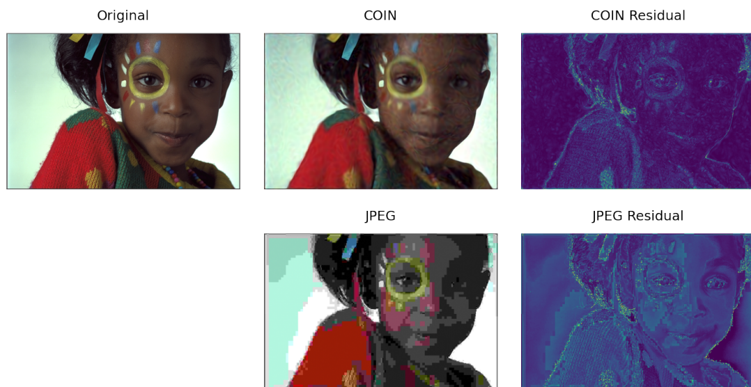
Figure 3.11: Comparison between COIN and JPEG on image 15 at 0.15bpp. The PSNRs are 27.35dB and 21.74dB respectively.
