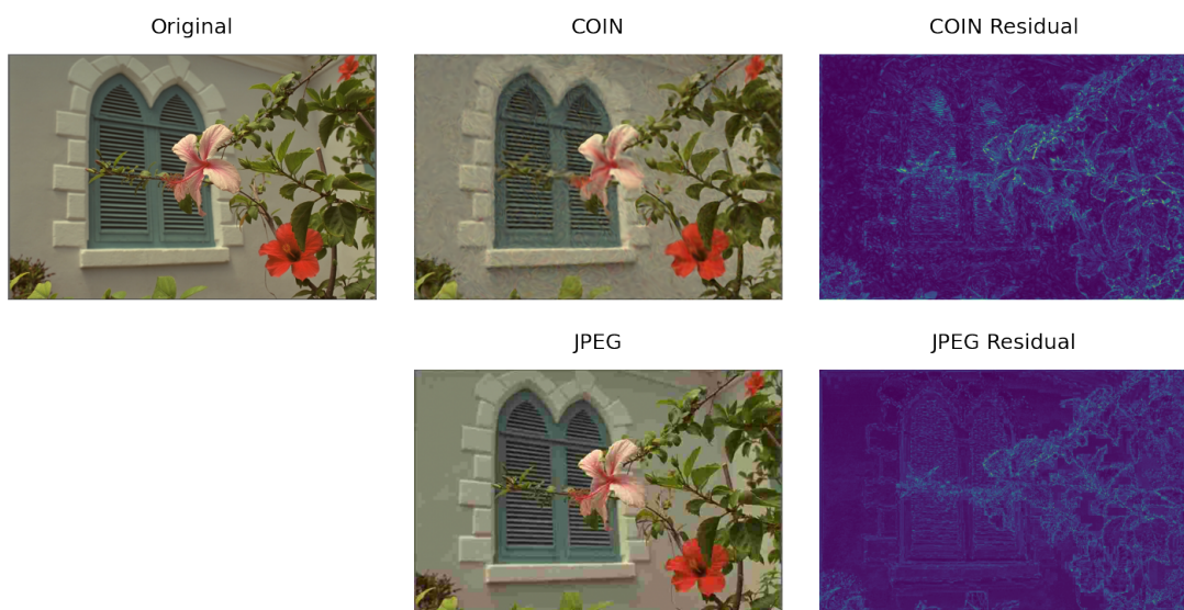
Figure 3.10: Comparison between COIN and JPEG on image 7 at 0.3bpp. The PSNRs are 26.92dB and 27.56dB respectively.
