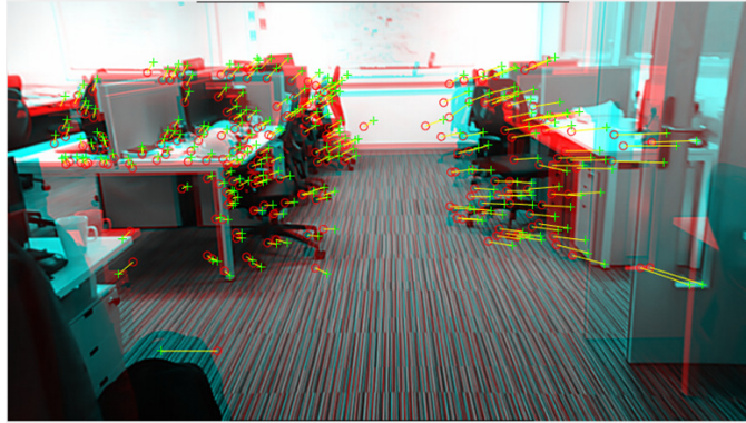
Figure 2.1: An example of feature extraction and matching process using SURF features and descriptor.
