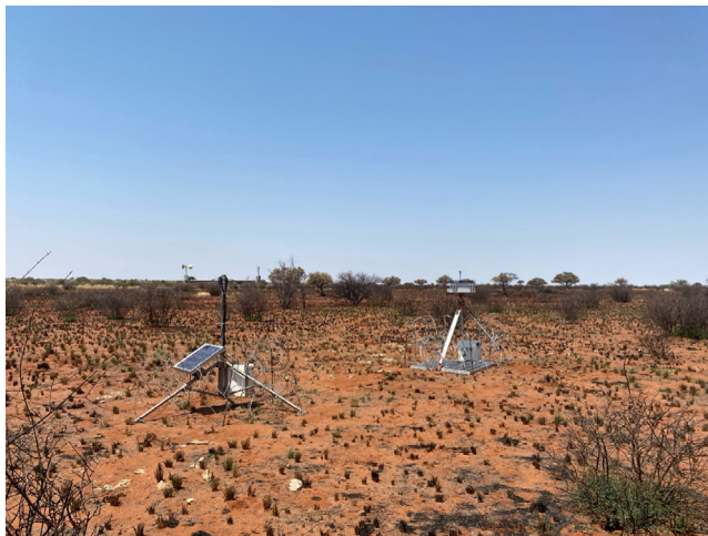
FIGURE 2 In-situ measurements of dust using a DustTrak monitor and meteorological station at site K02 burned interdune in September 2022.
