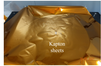
(c) 40 layers of 0.025-mm-thick Kapton sheets provide further insulation by minimising the probability of a current breakdown.
