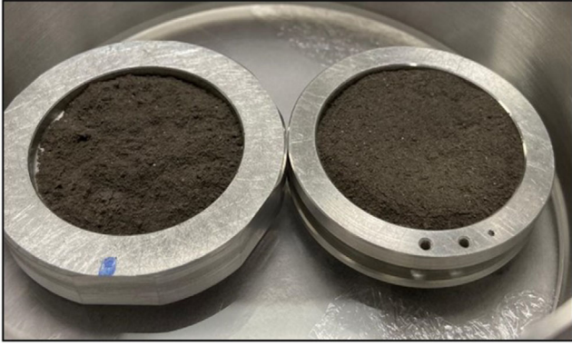
FIGURE 1. Left: A “rough” Apollo 16 (68810) sample used in the VOSEG physical property variation study. Right: A “smooth” Apollo 16 (68810) sample used in the VOSEG physical property variation study.
