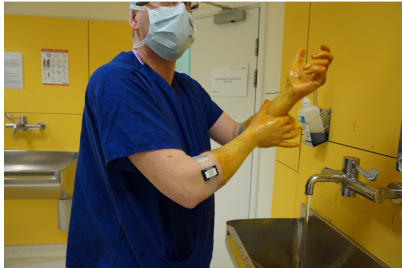
Figure 3.1: Wireless elbow-worn motion sensors being used while scrubbing before an arthroscopic procedure
