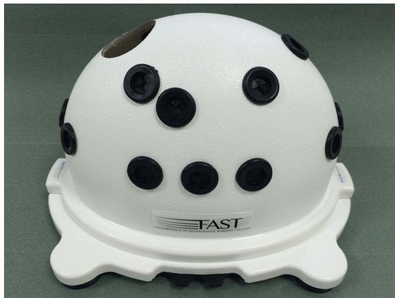
Figure 3.12: External view of the FAST workstation generic arthroscopy simulator. The tasks inside are modular and can be exchanged.
