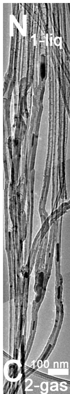
Figure A20. TEM images of several MWCNTs with junctions obtained by the liq/gas approach showing a change in structure from the N_{1\text{-liq}} section (bamboo-like structure) to the C_{2\text{-gas}} section (thicker walls). The image was obtained from different TEM images taken at the same magnification. The darker features are metal catalyst particles within the nanotubes.
