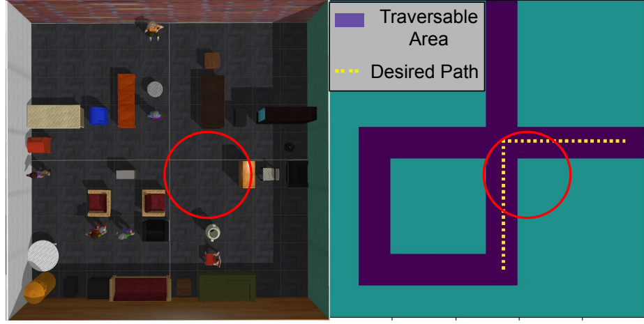
Figure 5.4: An example of randomised environments in ROS Gazebo and its map. An oracle commander is designed accordingly to give the robot correct commands before it reaches the turning and termination point. The red circle highlights a challenging situation where the intersection is not fully constrained with obstacles which can easily confuse the robot.
