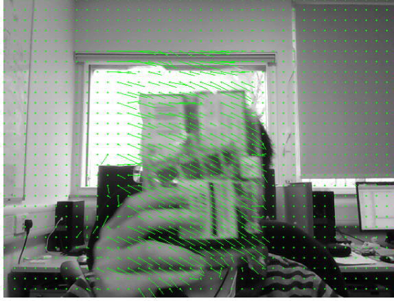
Figure 2.6: Output of optical flow. The green arrows display the direction of moving pixels while the dots represent the static ones.
