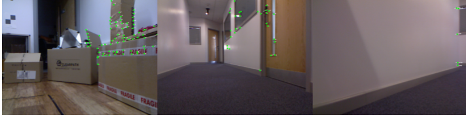
Figure 3.9: The left image is the feature detection result in the cluttered environment and the remaining two are in the corridor environment.
