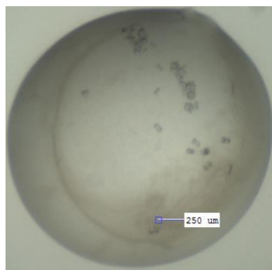
Figure 3-19. Crystals formed in a drop from crystal plates set up with co-expressed MRPP1-MRPP2 protein complex. Condition: 50% PEG200, 0.2 M \text{MgCl}_2 , 0.1 M cacodylate pH 6.5 grew after 3 days of incubation.
