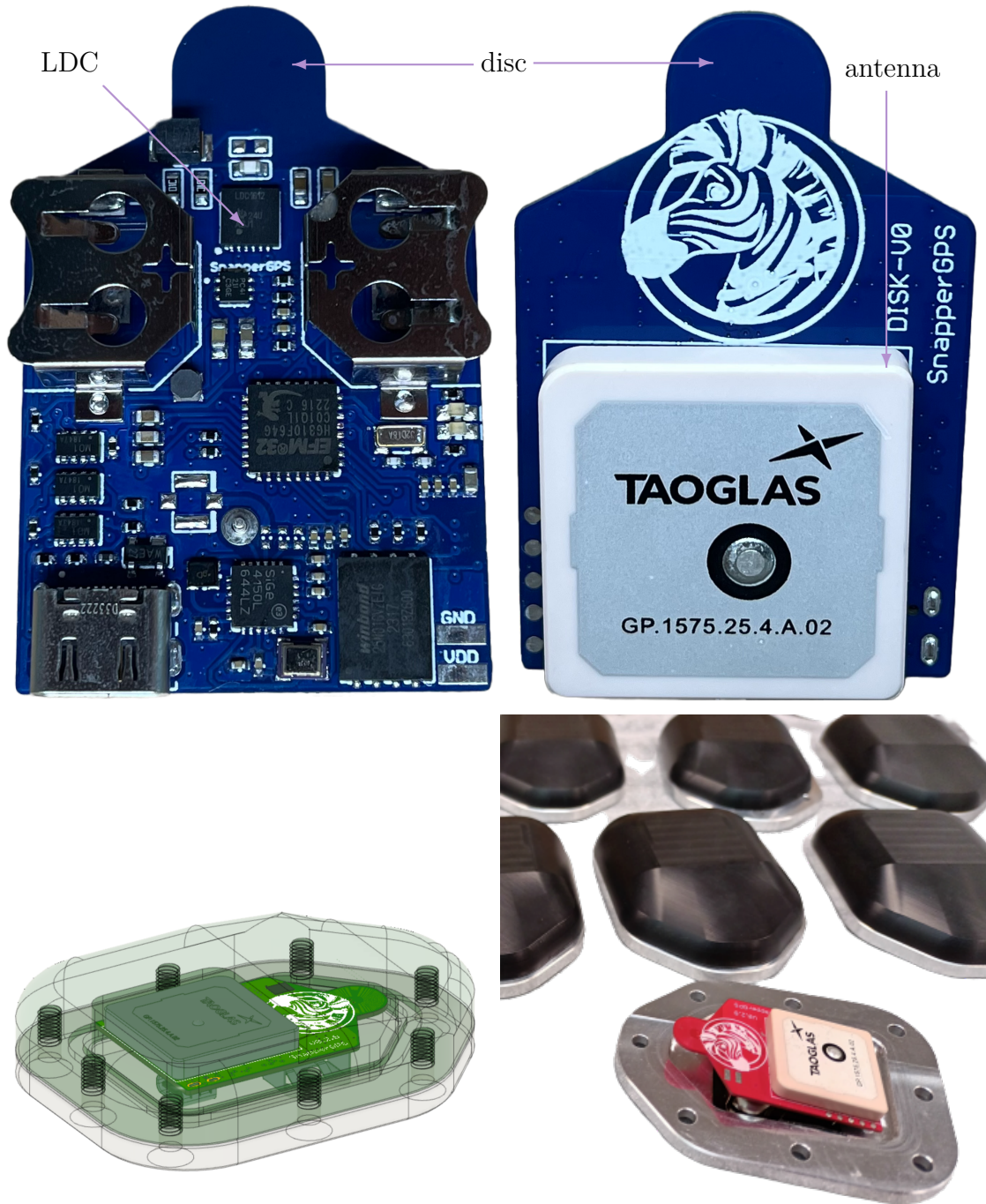
Figure 4.14: Top-left: Bottom view of a SNAPPERGPS board with integrated copper disc and LDC at the top. Top-right: Top view of the same board with an integrated passive patch antenna. Bottom-left: 3D model of the board in a custom enclosure. Bottom-right: Custom CNC-milled enclosures made of POM with an o-ring for sealing. The enclosures have a low profile to minimise drag and are pressure tested to be waterproof at 12 bar, which corresponds to about 120 m water depth.
