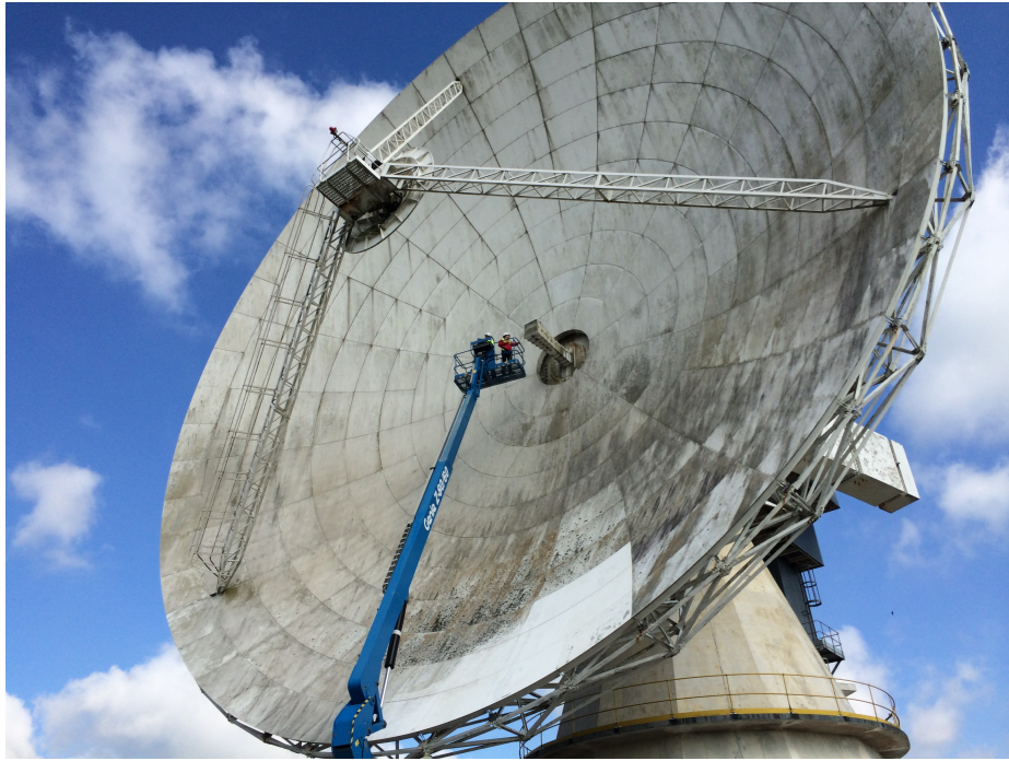
Figure 2.6: Verification of the antenna model by measuring the distance between the secondary and primary vertex.
