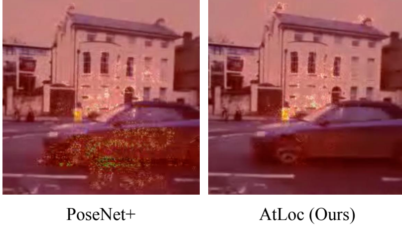
Figure 3.1: Response maps of one scene selected from Oxford RobotCar [174] indicate that AtLoc is able to force the neural network model to focus on geometrically robust objects (e.g. building structures in the right) rather than environmental dynamics (e.g. moving vehicles in the left) compared with PoseNet+ [28].
