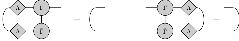
Figure 3.14: We show the condition for an iMPS to be in canonical form. This is the case if, at any bond, the transfer operator constructed from the \Gamma and \Lambda matrices satisfy both of these conditions (i.e., the identity is both a left and right eigenvector of the transfer operator)
