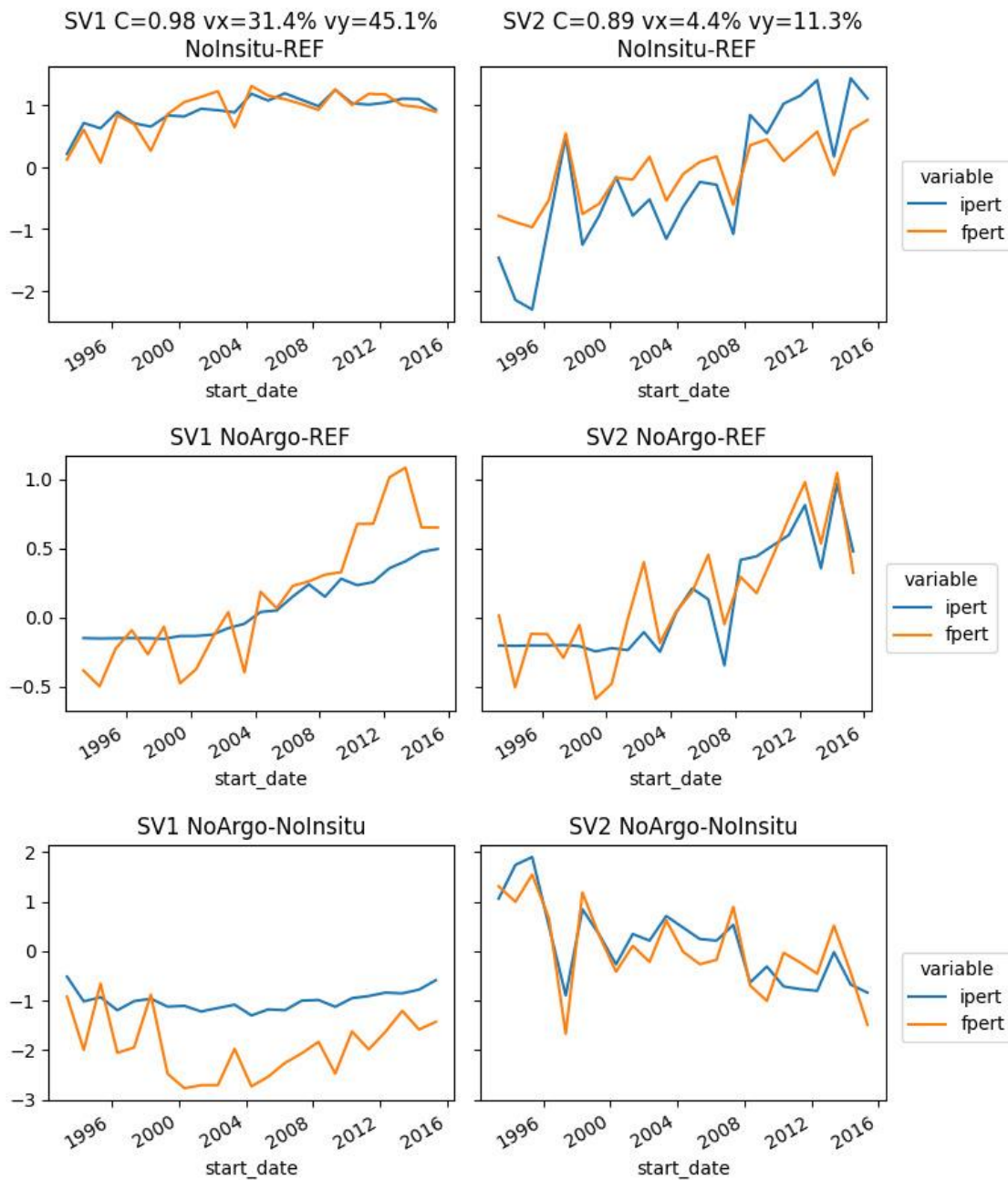
Supplementary Figure S8. Time series of first (left) and 2nd (right) modes of the singular value decomposition between \delta F_c and \delta I_{ni} . The time series are those shown in Fig 5 of the main text, but the generic sample time has been disaggregated into the contribution from the different OSE experiments.
