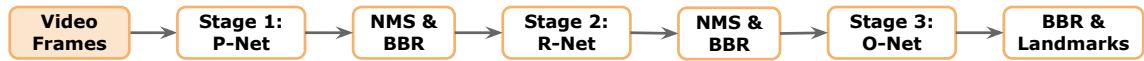
Figure 3.5: Steps of face detection. NMS: non-maximum suppression. BBR: bounding box regression. It includes three sub-networks (P-Net, R-Net and O-Net) in different detection stages. The detected facial images by O-Net are then used as the input (biometric samples) to SCAN.
