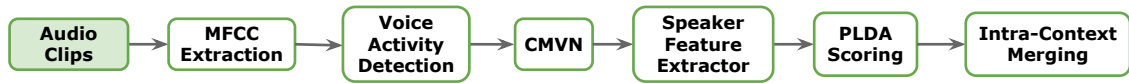
Figure 3.4: Steps of utterance segmentation. MFCC: Mel-frequency cepstral coefficients; CMVN: cepstral mean and variance normalization; PLDA: probabilistic linear discriminant analysis. The speaker feature extractor used in this implementation is x-vector [3]. Segmented utterances are then used as the input (biometric samples) to SCAN.
