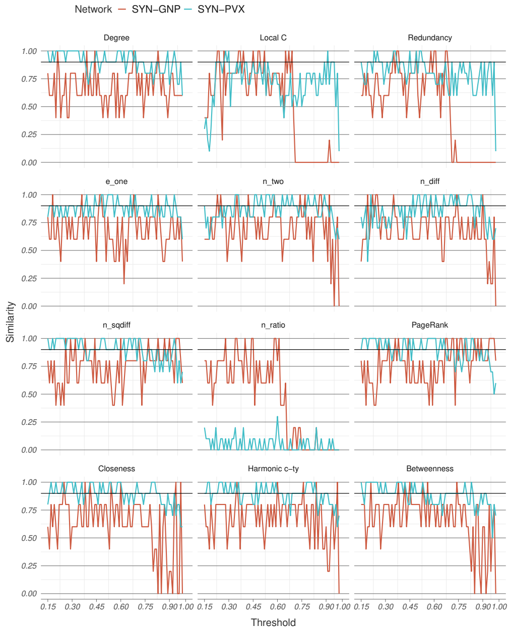
Figure A.3: Standard metric rank similarity between consecutive thresholds for the synthetic networks. The Bernoulli synthetic network, SYN-GNP, exhibits consistently lower similarity across all node metrics aside from the ratio between the step-1 and step-2 ego networks (n_ratio).
